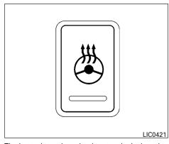
The heated steering wheel system is designed to operate only when the surface temperature of the steering wheel is below approximately 68°F (20°C).
